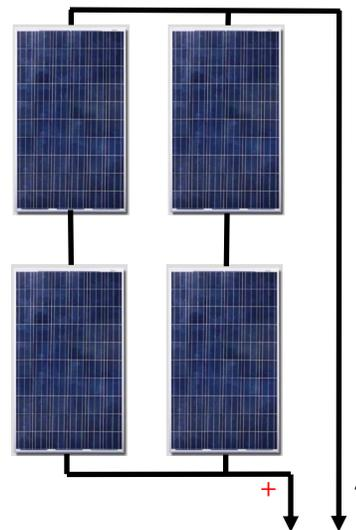
Four 36 cell Panels at up to 140 Watts
