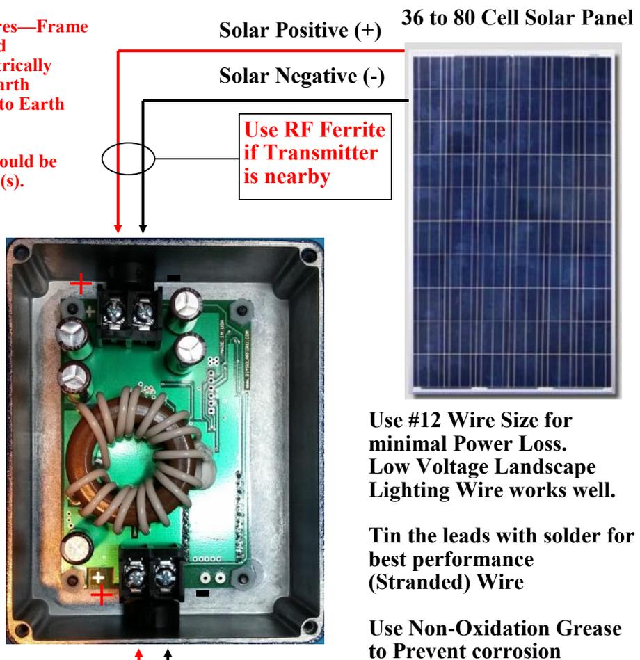
Connect Additional Charge Controllers in the same manner using one circuit breaker for each. Breaker output from each connects to Battery (+) Terminal.
